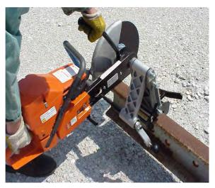
Mounting the Ultra Kut III Saw
