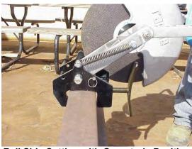
Rail Side Cutting with Operator's Position
