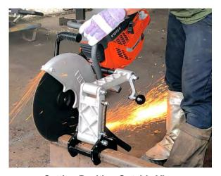
**Cutting Position Outside View**Pivot shaft and thread engaging tightening crank.
